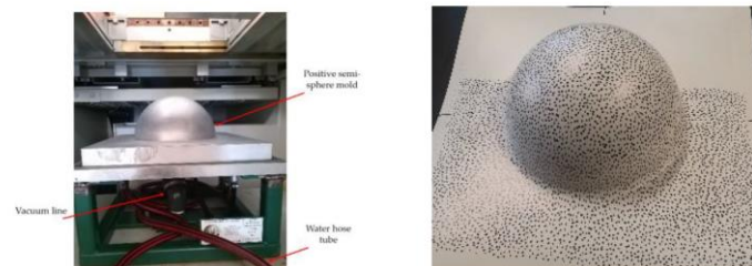
Figure 1: Semi sphere, D250mm, thermoforming mould (left), thermoformed product with DIC spackle pattern (right)
